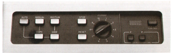
Fig. 6. Control panel of the 4700A. The recording function is selected by using the keys on the left and the format can be selected and/or modified by using the display, keys, and rotary switch on the right.
