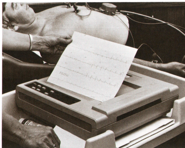
Fig. 1. The HP Model 4700A PageWriter Cardiograph is a state-of-the-art machine that records ECG data in a page-sized format with high trace quality. The page format makes it easier to interpret ECG data and file it for future reference.
